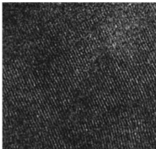
Figure 8. TEM micrograph of [\text{Pt}(\text{NH}_2\text{R})_4][\text{PtCl}_4] , with R = heptyl.
