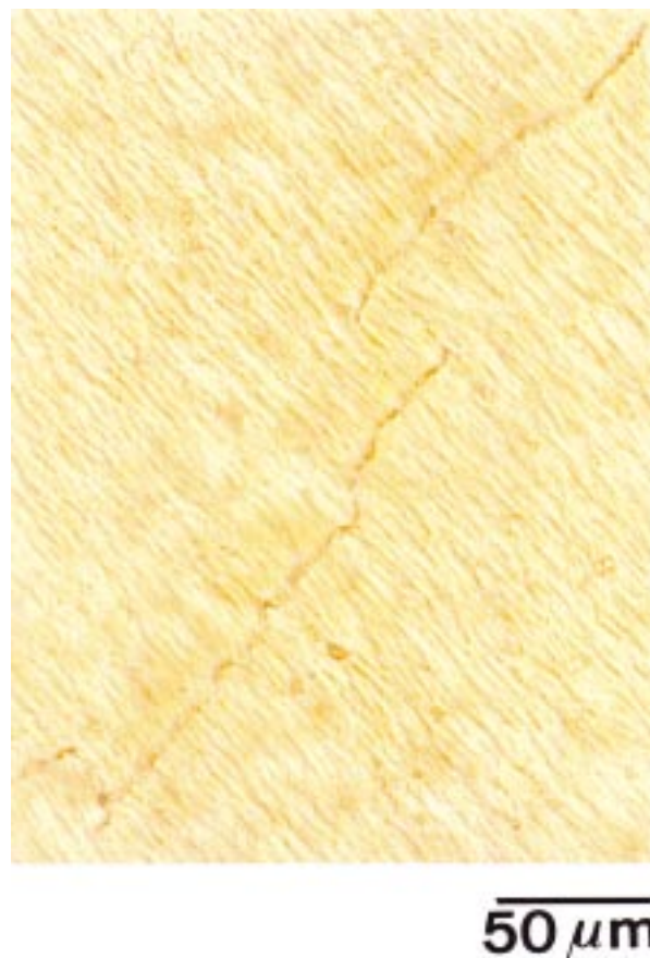
Figure 12. Film of [\text{Pt}(\text{NH}_2\text{R})_4][\text{PtCl}_4] , with R = octyl, prepared by mechanical drawing in the gel state followed by solvent evaporation, imaged under crossed polarizers with an optical microscope. The drawing axis is oriented 45° to the polarization axes of the polarizers.
