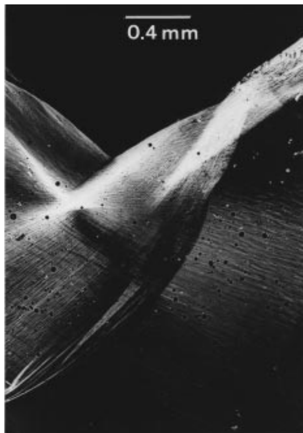
Figure 9. Gel of [Pt(NH_2R)_4][PtCl_4] , with R = heptyl, in CHCl_3 imaged between crossed polarizers with an optical microscope.
