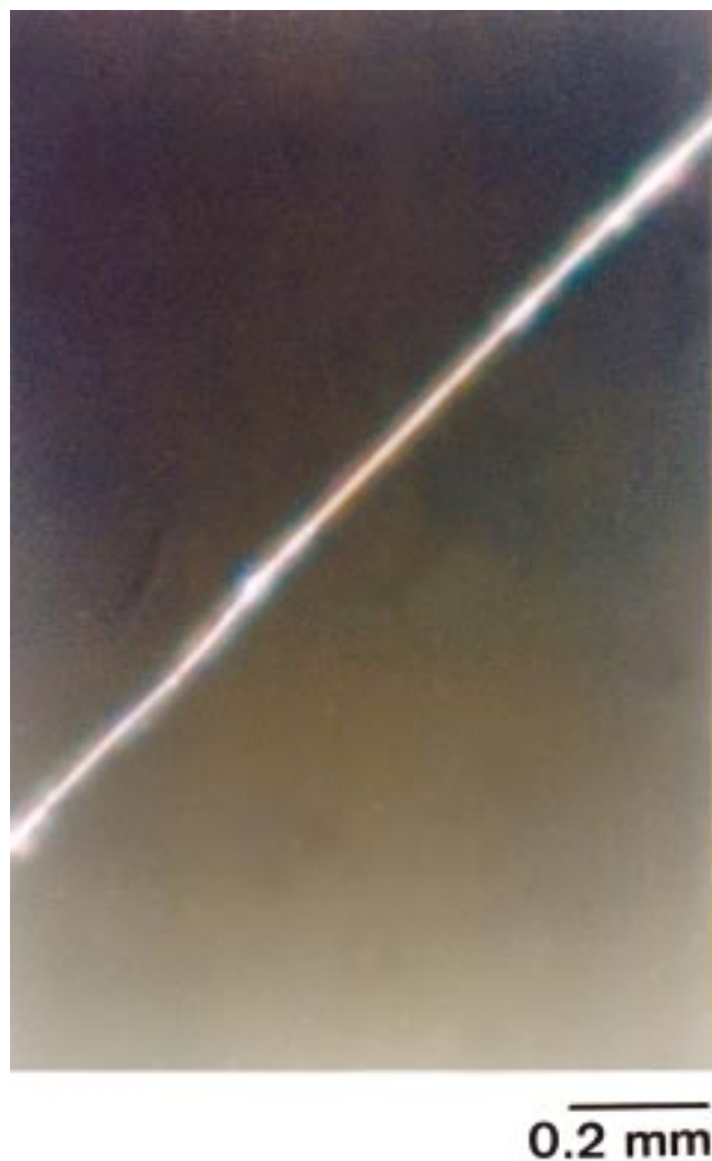
Figure 13. Fiber of [\text{Pt}(\text{NH}_2\text{R})_4][\text{PtCl}_4] , with \text{R} = \text{octyl} , prepared by electrostatic spinning, imaged under crossed polarizers with an optical microscope. The fiber axis is oriented 45^\circ to the polarization axes of the polarizers.
